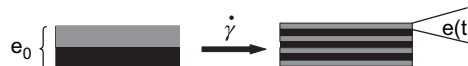
Fig. 9. Simplified vision of laminar mixing with decrease of the striation thickness, \delta = e_0/2 in simple shear flow.
